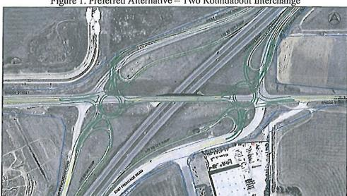
Figure 1. Preferred Alternative - Two Roundabout Interchange
